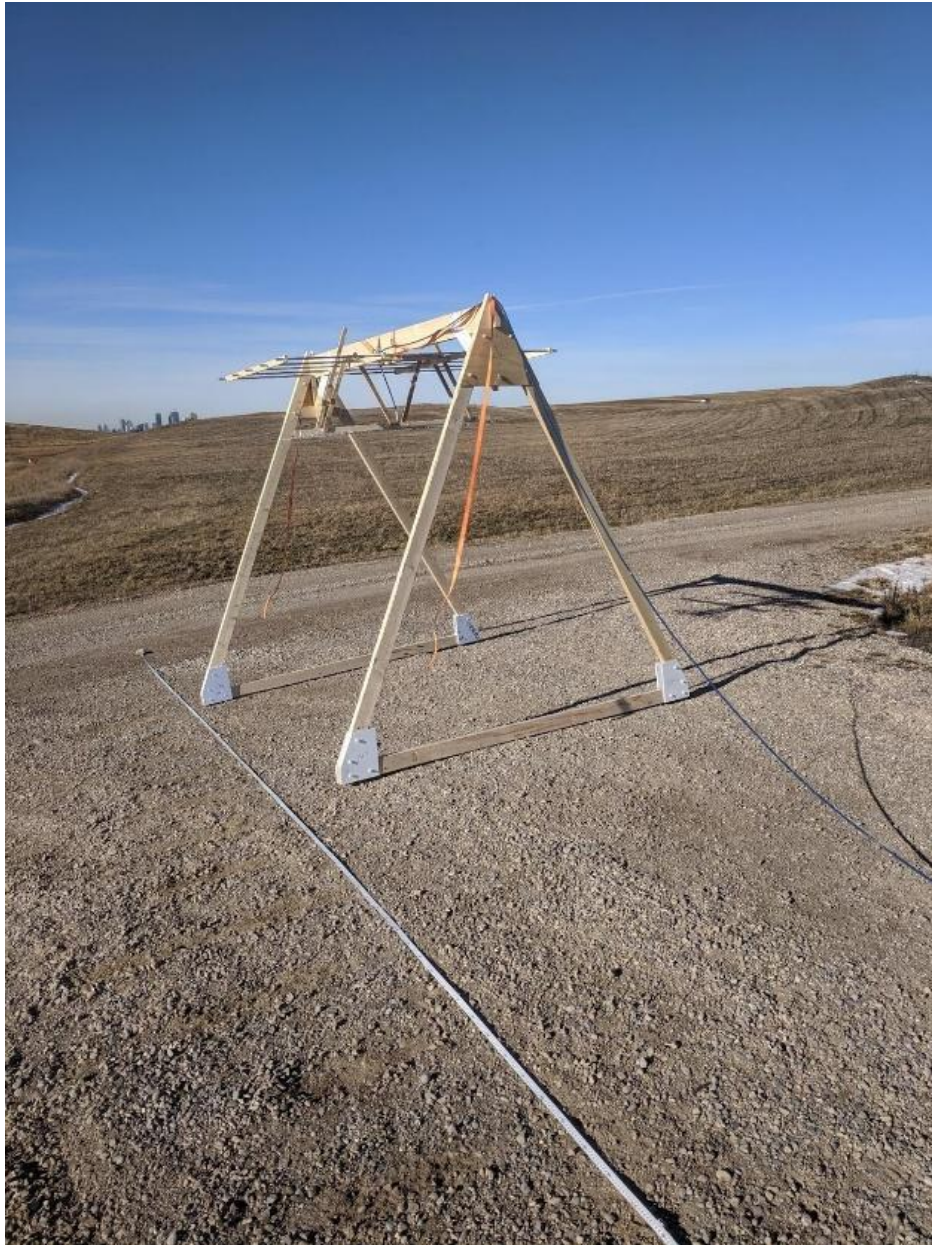
Figure 10 – Prototype hardware to simulate drone sensor data collection
