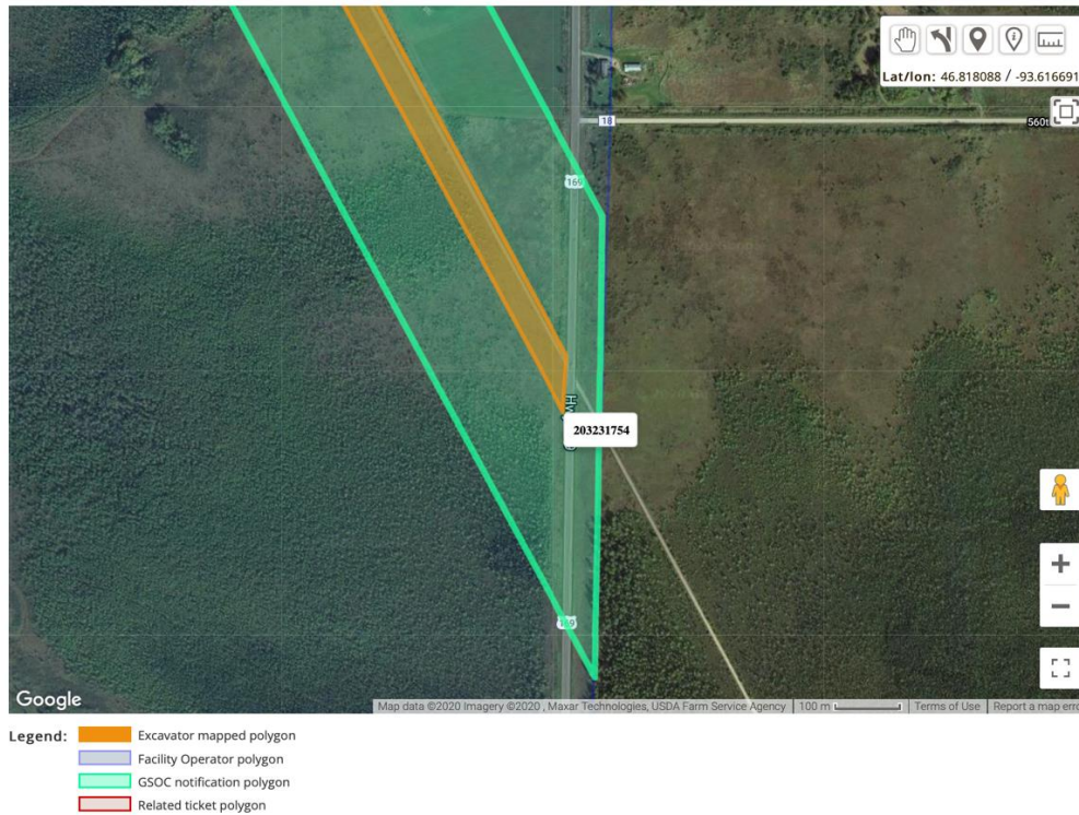
Figure 8 – Locator sees where proposed excavation areas overlap with underground gas facilities
